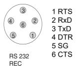
1 Connect the RS232 interface to the external printer with the AK540/ S cable.
