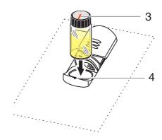
3 Align the cell marking (3) with the marking (4) of the cell shaft. The cell is ready to be measured.
